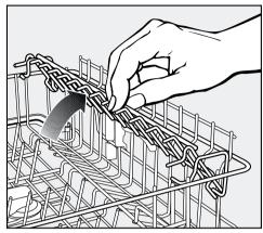
The adjustable cup rack can be raised to make room for taller items or lowered to double stack smaller items.
